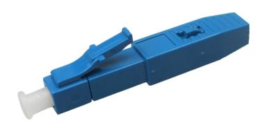
LC quick assembly connectors connectors are factory terminated and polished to make fibre terminations fast, easy and reliable. These fibre optic connectors offer terminations in less than 2 minutes without any difficulty and require no epoxy, polishing or crimping. They greatly reduce the installation and set up time. It has a window feature to allow testing with a visual fault locator.
