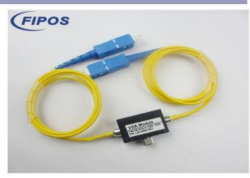
The variable attenuator is a kind of fiber optic attenuator that supports continuous adjustment of attenuation value between 0.6dB and 60dB. It employs the principle of light shading between the two collimators to control the attenuation value by a knob that can be manually rotated. This range of variable optical attenuator offers adjustment accuracy up to 0.1dB.
