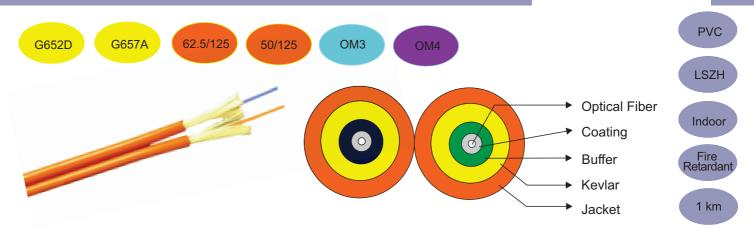
Optronics zip duplex fiber optic patch cable is constructed with two simplex units joined together with a central web. Ideal for use in office LAN connections, patchcords, pigtails and internal point-to-point links where frequent handling is likely (e.g. data cabinets, equipment rooms, user outlets). Utilising 600µm or 900µm buffered fiber, the cable is suitable for use with industry standard connectors and can be easily made into a patchcord.
