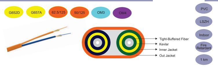
Optronics flat duplex fiber optic patch cable is constructed with two simplex units held together with an overall PVC/LSZH jacket. Ideal for use in office LAN connections, patchcords, pigtails and internal point-to-point links where frequent handling is likely (e.g. data cabinets, equipment rooms, user outlets). Utilising 900µm buffered fiber, the cable unit is suitable for use with industry standard connectors and can be easily made into a patchcord.
