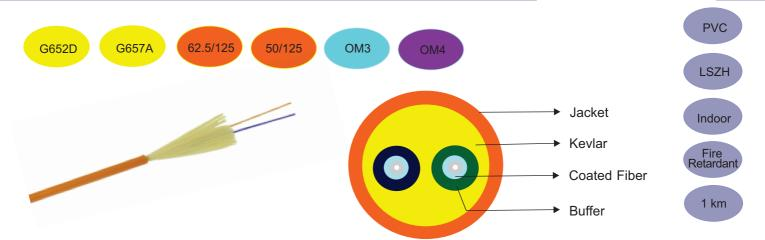
Optronics round duplex fiber optic patch cable is constructed with two tight buffered fibers protected by aramid yarns and an PVC/LSZH jacket. Ideal for use in office LAN connections, patchcords, pigtails and internal point-to-point links where frequent handling is likely (e.g. data cabinets, equipment rooms, user outlets). Utilising 600µm or 900µm buffered fiber, the cable unit is suitable for use with industry standard connectors and can be easily made into a patchcord.
