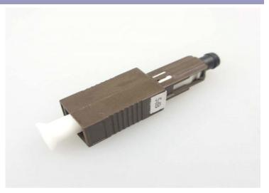
Fiber optic attenuators are used in the fiber optic communications to reduce the optical fiber power at a certain level, the most commonly used type is female to male plug type fiber optic attenuator. Plug type MU attenuator has the optical fiber connector at one side and the other side is a female type fiber optic adaptor.
