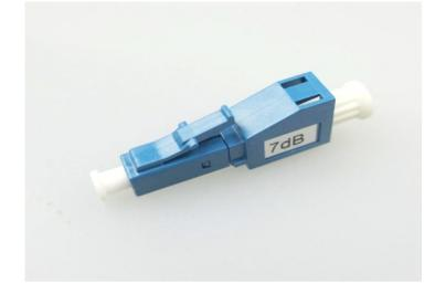
Fiber optic attenuators are used in the fiber optic communications to reduce the optical fiber power at a certain level, the most commonly used type is female to male plug type fiber optic attenuator. Plug type LC attenuator has the optical fiber connector at one side and the other side is a female type fiber optic adaptor.
