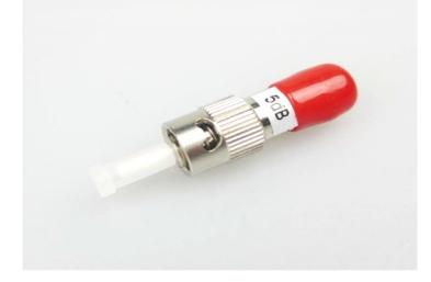
Fiber optic attenuators are used in the fiber optic communications to reduce the optical fiber power at a certain level, the most commonly used type is female to male plug type fiber optic attenuator. Plug type ST attenuator has the optical fiber connector at one side and the other side is a female type fiber optic adaptor.
