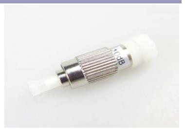
Fiber optic attenuators are used in the fiber optic communications to reduce the optical fiber power at a certain level, the most commonly used type is female to male plug type fiber optic attenuator. Plug type FC attenuator has the optical fiber connector at one side and the other side is a female type fiber optic adaptor.
