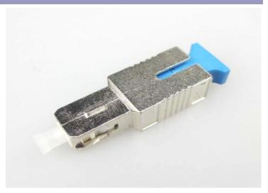
Fiber optic attenuators are used in the fiber optic communications to reduce the optical fiber power at a certain level, the most commonly used type is female to male plug type fiber optic attenuator. Plug type SC attenuator has the optical fiber connector at one side and the other side is a female type fiber optic adaptor.
