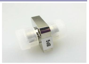
Adaptor-type attenuator has the same appearance as regular fiber optic adaptor. It achieves attenuation of optical signal by setting up an attenuation film inside a fiber optic adaptor to ensure incomplete touch with fiber connectors. The attenuator is a great fiber optic attenuation solution for fiber patch cords in a optical link.
