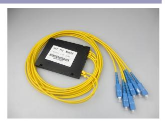
Planar Lightwave Circuit (PLC) Splitter is a type of optical power management device that is fabricated using silica optical waveguide technology. It features small size, high reliability, wide operating wavelength range and good channel-to-channel uniformity, and is widely used in EPON networks to realize optical signal power splitting.
