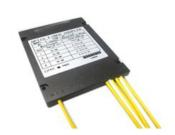
FBT Coupler Splitters is widely accepted and used in passive optical networks, especially for instances where the split configuration is smaller (1×2, 1×4, etc.). FBT is the traditional technology in which two fibers are placed closely together, typically twisted around each other and fused together by applying heat while the assembly is being elongated and tapered. Our supply high quality FBT splitters with single/double/three windows .
