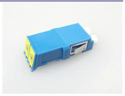
LC shuttered adaptors is designed specifically to prevent end surface damage of the ferrule. It has a high precision zirconia alignment sleeve designed for high reliability and excellent reconnectability in all singlemode networks. It has an spring loaded plastic shutter for laser safety and dust protection.
