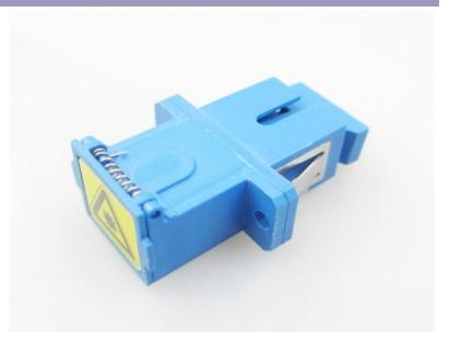
SC shuttered adaptor integrates safety features suitable for FTTH and other telecom applications. It has a high precision zirconia alignment sleeve designed for high reliability and excellent reconnectability in all singlemode networks. It has an spring loaded plastic shutter for laser safety and dust protection.
