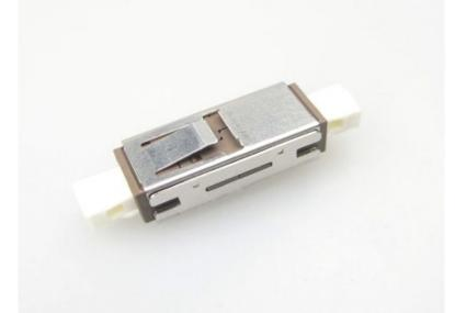
Adaptor is a mechanical device designed to align fiber optic connectors. It contains the interconnect sleeve that holds two ferrules together. Our MU fiber adaptor are at least half the size of the standard SC adaptor. They offer twice the port density, a new solution for high performance telecommunications networking.
