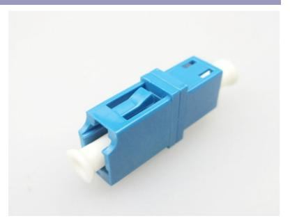
Our range of LC adaptor have high precision alignment sleeves for improved reliability and better reconnectability. The LC adaptors come with ceramic sleeves for both singlemode and multimode. The housing is available in different colors with options for flange or flangeless body.
