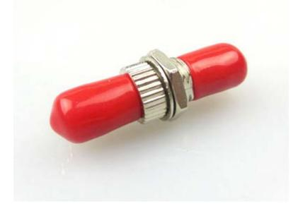
Our ST adaptor have high precision alignment sleeves for reliability and better reconnectability. ST adaptors come with a ceramic sleeve for the singlemode adaptor and phosphor bronze sleeve for the multimode adaptor.
