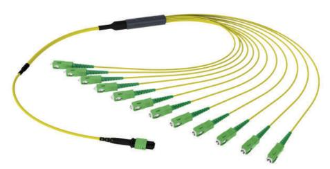
MTP/MPO Ruggedised Fan-Out Assemblies route multifiber MTP/MPO connection into discrete connectors. They are used to directly interconnect MTP/MPO cassettes, panels or backbone assemblies with the active equipment, saving costly data center rack space and easing fibre management. MTP/MPOFan-Outs are built with highest quality components. Standard MTP/MPO as well low loss Elite versions are offered featuring low insertion loss for demanding high speed networks where power budgets are critical.
