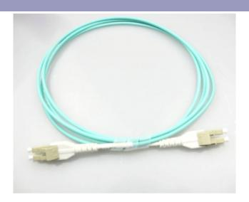
Our uniboot fibre patch cord reduces cable management space by up to 68% compared to standard patch cords. The patch cord utilises a special "round duplex" cable that allows duplex transmission within a single 3mm or 2.4mm cable. As a result of these features our uniboot patch cord offers improved airflow and visibility of equipment within a high density network environment.
