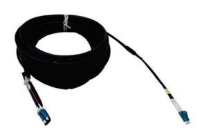
FTTA RRU armored outdoor fiber patch cord is used for fiber to the antenna, and duplex base station far transmission fiber optic patch cable is kind of indoor/outdoor patch cord, built on LSZH cables with 7.0mm or 4.8mm diameter, with water blocking aramid yarns and UV resistant black out jacket.
