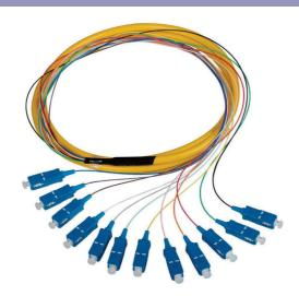
Bundle Fan-out Fiber Optic Pigtail is a piece of fiber optic cable with only one fiber optic connector on one side of the cable, there are singlemode and multimode fiber optic pigtails. They typical use is to link the fiber optic cable with fiber optic equipment, while the other side of the pigtail is melted together with the fiber cable, by melting together the fiber glasses, it can reach a minimum insertion loss.
