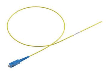
G657 Bend-insensitive singlemode pigtails exhibit much lower optical power loss under bend conditions while remaining compatible with conventional cabling. They are designed to reduce optical loss when the cable is bent. G657 Bend-insensitive singlemode pigtails provide the same high quality, mechanical features and optical performance as our standard pigtail with the added capability of maintaining optical performance when bent or flexed.
