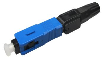
SC fiber optic fast connectors are factory terminated and polished to make fibre terminations fast, easy and reliable. These fibre optic connectors offer terminations in less than 2 minutes without any difficulty and require no epoxy, polishing or crimping. They greatly reduce the installation and set up time. It has a window feature to allow testing with a visual fault locator.
