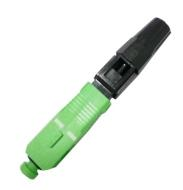
SC/APC fiber optic fast connectors are factory terminated and polished to make fibre terminations fast, easy and reliable. These fibre optic connectors offer terminations in less than 2 minutes without any difficulty and require no epoxy, polishing or crimping. They greatly reduce the installation and set up time. It has a window feature to allow testing with a visual fault locator.
