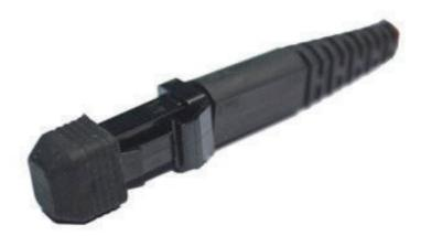
MT-RJ is a fiber-optic Cable Connector that is very popular for small form factor devices due to its small size. Its size is slightly smaller than a standard phone jack and just as easy to connect and disconnect. Housing two fibers and mating together with locating pins on the plug, the MT-RJ comes from the MT connector, which can contain up to 12 fibers.
