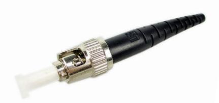
The ST connector was originated by AT&T Bell Laboratories for use in premises wiring of buildings and other applications. Thanks to its simplified one-piece design, it is the most popular 2.5mm ferrule connector for field assembly. Available in singlemode and multimode, the ST style connector is a low cost and reliable connection solution in the industry.
