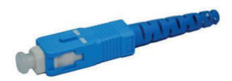
The SC connector is another popular type of 2.5mm ferrule connector. Compatible with NTT push/pull SC connectors, the pre-assembly plug body provides easy and quick termination. With the plastic clip, two simplex connectors can clip together and form a duplex connector. A wide range of SC connectors are available in stock.
